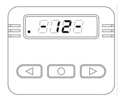
If the Temperature Control mode is selected (regardless of activation of the Ventilation mode), then the required value of temperature is set by pressing the buttons (decrease) or (increase)
